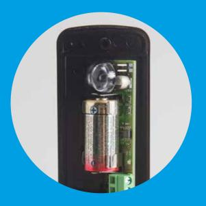
To minimize wired interventions and further simplify installation operations, the DXR range also features a version with battery-powered transmitter, with a duration of up to 24 months\*, infrared range adjustable from 5 to 10 meters and the possibility of synchronizing up to 2 pairs of photocells. In addition to the functions already available
