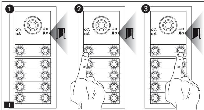
During call programming **I** ①, you can control the brightness and colour of the unit backlight. Press the left call button to select white **I** ②, and the right call button to select blue **I** ③.
