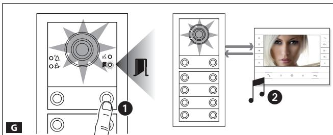
On the entry panel, press the call button to be linked to the internal receiver **G 1**. A beep confirms that the setting has been stored **G 2**. **2**. End the call and repeat for the other internal receivers.
