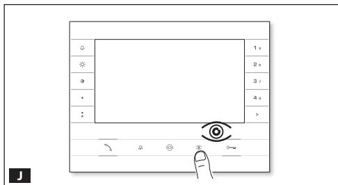
While programming the calls, the “visual range” of the video camera can be adjusted from any receiver. To do this, lift the handset (where present) and press the “self-connection” button **J**.
