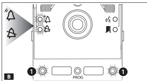
Press the first call button on each unit **C D** (see "Button numbering" section) until the blue LED  $\Delta$  and the button LEDs stop flashing.
