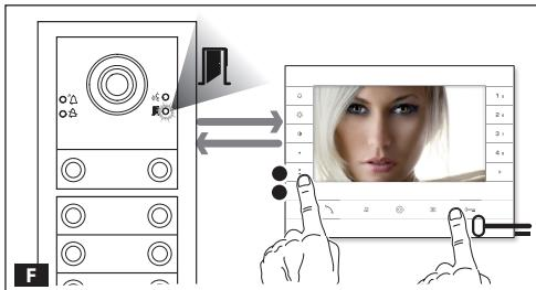
The green LED flashes. Lift the internal receiver handset (if present) and press the door lock release and AUX2 buttons **F**.
