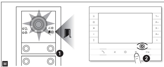
While programming calls **M ①** the brightness level of the entry panel can be adjusted from any receiver. Pressing the “self-connection ” button on the internal receiver **M ②** activates the video camera on the entry panel for which the brightness level is to be adjusted.
