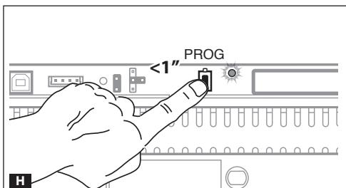
Press the PROG button briefly **H**. The LEDs on the entry panel switch off.
