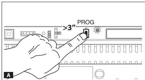
Press the PROG button on the power supply **A** until the PROG LED lights up.
