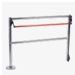
Safety barrier made of AISI 304 stainless steel with panic push-bar. Available with either left or right-hand column. L = 900 or 1200 mm, H = 1000 mm.
