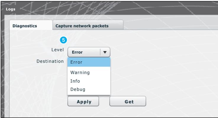
It is possible to choose the type of error **5** to be filtered, whether to store the log files locally in the device's memory **6** or in a Syslog specifying the IP address **7**.
