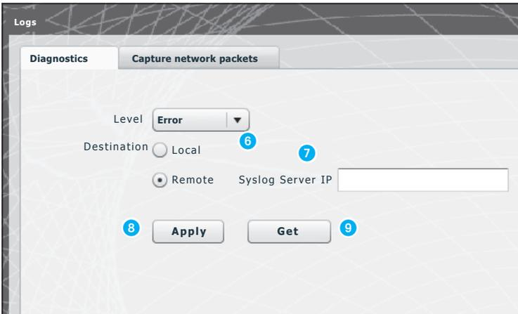
By pressing the "Apply" button **8** it is possible to apply the set-up selected once it is changed.
