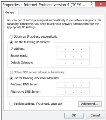
The entry "**Use the following IP address**" appears on this screen and you should fill in the fields as follows:
