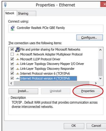
From the "**Ethernet Status**" window select "**Properties**"; highlight the heading "**Internet Protocol version 4 (TCP/IPv4)**" and click on "**Properties**".
