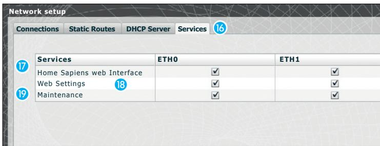
The section '**Services**' **16** is only available if the configuration of the two gateways is Dual Network. For each gateway it is possible to enable or disable the services listed below:
