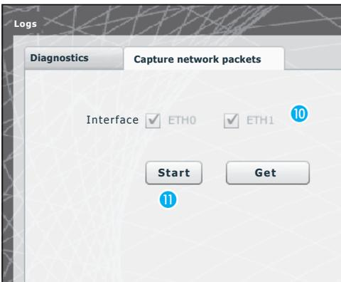
From tab "Capture network packets" it is possible to start gathering all the data that transmits from/to the device (**NOT the traffic that transits from one gateway to the other**).
