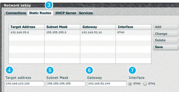
The **static routes** ③ are rules for transmitting IP packets to different networks than the two subnets corresponding to the ETH0 and ETH1 interfaces. This section is only present in Dual Network mode
