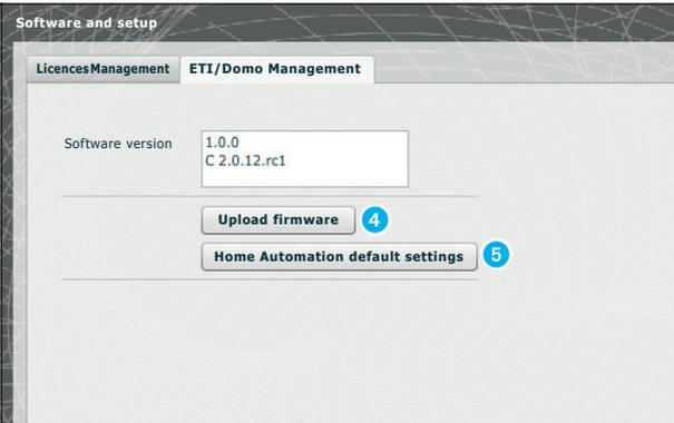
In the section “**ETI/Domo Management**” you can display and update the software version installed. Once the file for the update has been received, press button 4, select the file and proceed with the upload.
