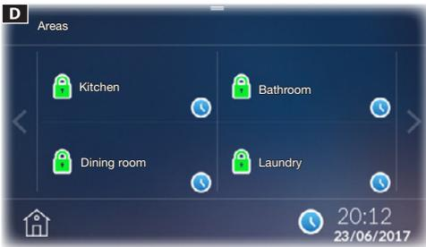
Enter the password; if the password is valid, you can access the screen **D** showing the list of areas and the status of the scenario has been run.
