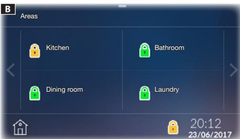
This screen allows you to view all the areas into which the alarm system has been divided. If you do not enter the authentication code, it is only possible to view the status of the areas and inputs that make them up.
