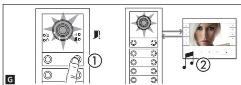
**NOTE.** The operation can only be carried out from the entry panel with the blue LED **A** off (1 entry panel in **F**). To change the entry panel from which calls are programmed, press one of the call buttons on the entry panel you wish to use for programming.
