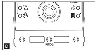
To enable the intercommunicating function, press the intercommunicating call button you want to call on the internal receiver you want to program **E**. A beep indicates that the function has been programmed successfully. Repeat for all internal receivers to be included in the intercommunicating group. To conclude the programming, press the PROG button on the entry panel briefly **F**.
