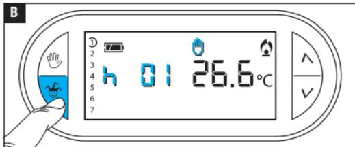
Press and use the buttons to set the desired activation times **B**.
