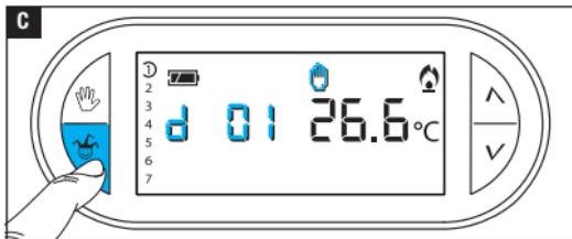
Press again and use the buttons to set the desired activation days **C**.
