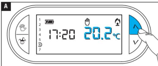
Use the  $\Delta$ / $\nabla$  buttons to adjust the desired temperature value **A**.
