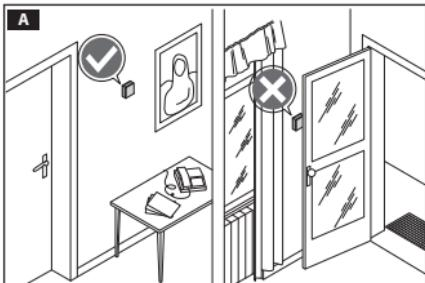
Install the unit in a suitable position to correctly detect the temperature, possibly in an internal wall, avoiding installation in niches, behind doors, curtains or near heat sources.
