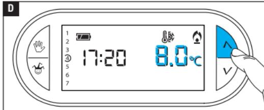
The **^**/**V** buttons can be used to set the minimum tolerated room temperature for the thermal zone.
