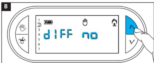
Use the **^****^** buttons to activate/deactivate the differential algorithm **B**.
