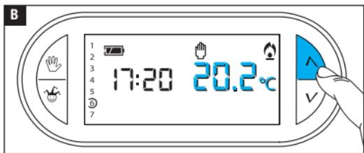
In addition to the current time, the display also shows the default manual temperature (20 °C).
