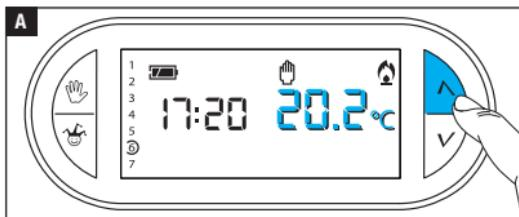
Use the **▲▼** buttons to set the desired temperature value **A**.
