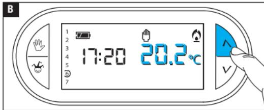
In addition to the current time, the display also shows the default manual temperature (20 °C).
