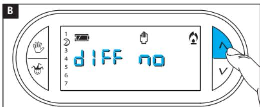
Use the  $\wedge \vee$  buttons to activate/deactivate the differential algorithm **B**.
