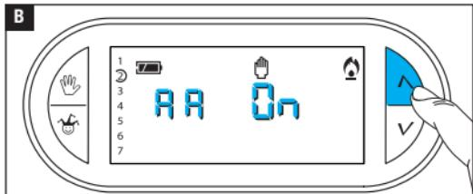
Use the  $\wedge \vee$  buttons to activate/deactivate the automatic advance **B**.
