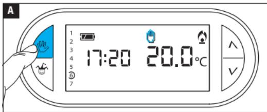
If you wish to temporarily disable automatic temperature control, you can switch to MANUAL operation by pressing **A**.
