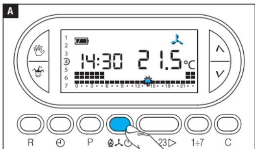
Press the button **A** to choose the operating mode for the thermal zone.
