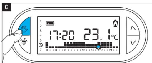
Using the  $1 \div 7$  button, move the indicator onto the chosen activation day **A**.
