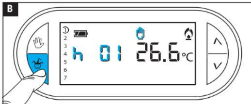
Press and use the buttons to set the desired activation times **B**.
