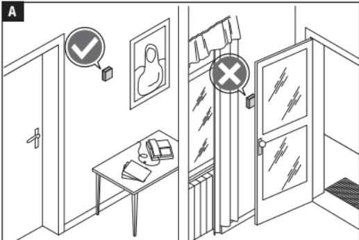
Install the device in a place suitable for detecting the room's temperature, possibly onto an inside wall, and avoid any nooks, behind doors, near curtains or heat sources.
