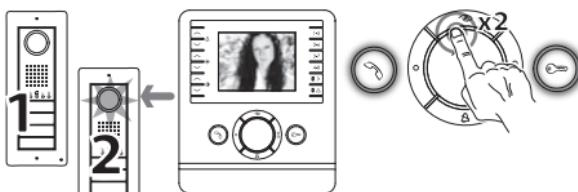
To end the communication, press the key twice or wait for the communication to end automatically (max. 60 seconds).
