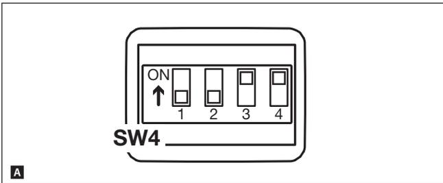
To restore module MTMRFID to factory settings it is necessary to disconnect the power supply, position DIP1 and DIP2 of SWITCH SW4 to ON and power the module again **A**.
