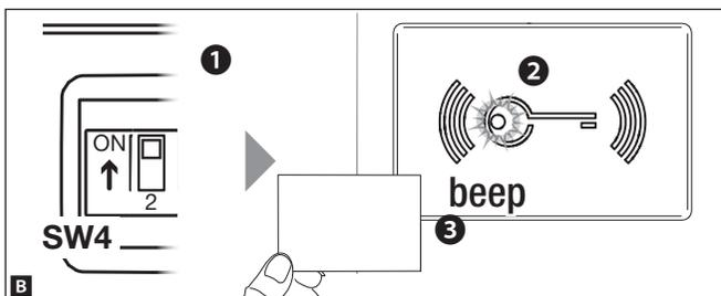
To remove badges from the associated relay, position DIP2 to ON **1**. When the red LED on module MTMRFID starts to flash quickly **2** swipe all the badges to be removed on the reader.
