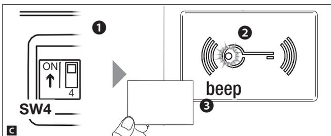
To remove lost badges, position DIP4 to ON **1**. When the red LED on module MTMRFID stays constantly on **2**, swipe all the badges previously acquired on the reader.
