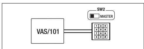
Use codes to access the programming functions. During a programming functions, the red light strip flashes every two seconds for an amount of times that corresponds the first digit of the programming code (when changing the password, the code is 10, and the light alert will flash once).
