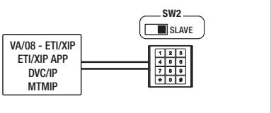
The sending of the device's ID code happens when you type the code **\* 0 0 0 #**.
